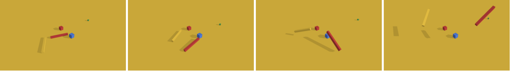
Fig. 3. A beam pinned between two posts as a block strikes at high velocity. Each frame shows the aftereffects of fracture for various values of \alpha (left to right): \alpha of 0, 0.5, 1, and 1.5. Larger values exaggerate the effect.
