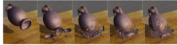
Figure 8: Comparison of vase impact at frame 190 with strain limits \tau = 0.01, 0.005, 0.001, 0.0005, 0.0002 decreasing from left to right.
