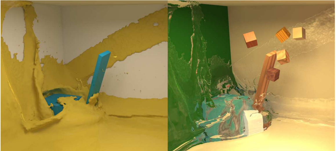
Figure 18: The left side of this figure is the computational domain, and the right is the rendered frame. On the left the yellow area is the fluid domain \mathbb{F} ; the blue is the rigid body domain \mathbb{R} . Notice that the small blocks on the right are not touching liquid, so they will be controlled by the rigid body solver until they touch liquid.
