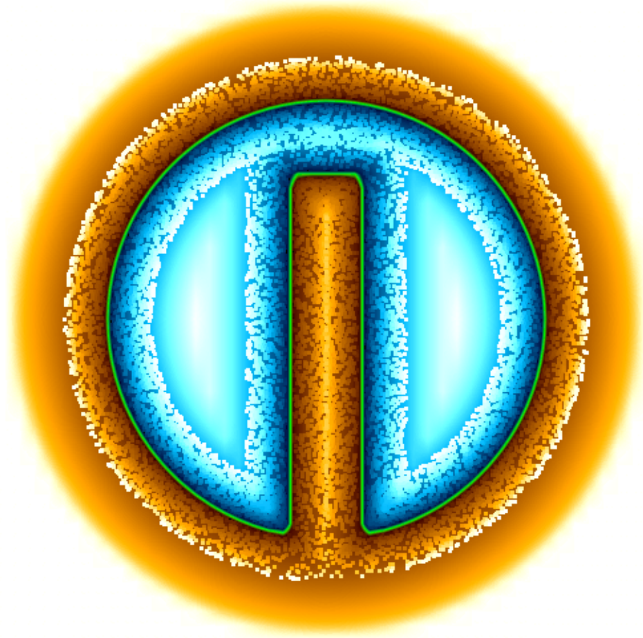
Figure 29: Lagrangian particles are placed on both sides of the level set in the particle level set method.
