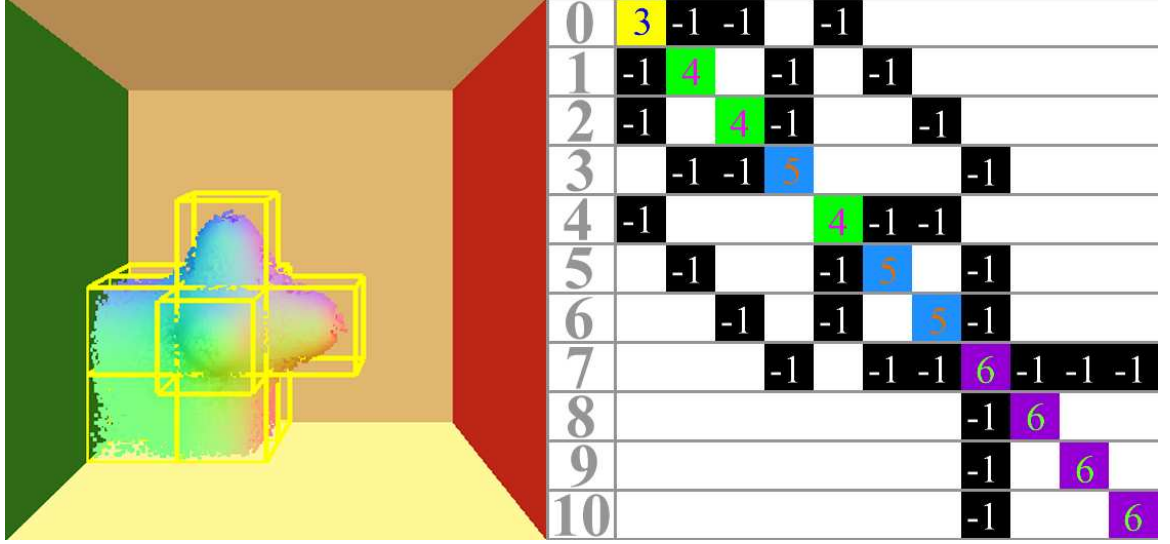
Figure 7: Fluid cells in a MAC grid (left), and the corresponding pressure projection matrix \mathbf{A} (right), and the indices into the array of fluid cells (center). The white matrix entries = 0.
